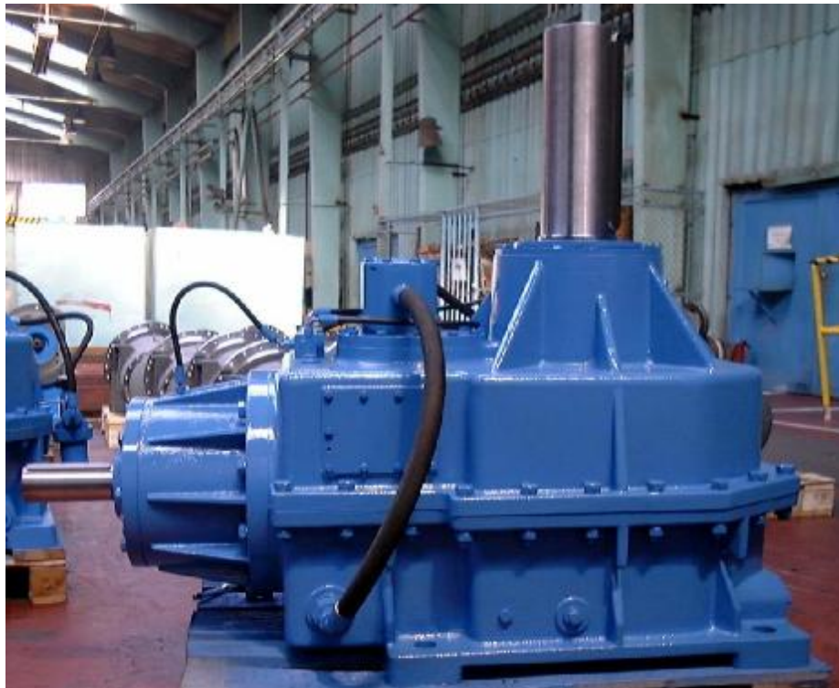
Gearbox KCV 12, power station Nasirija, Iraq
