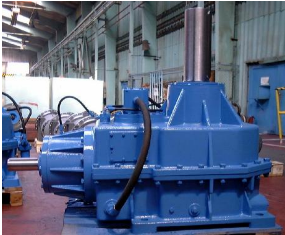
Gearbox KCV 12, power station Nasirija, Iraq
